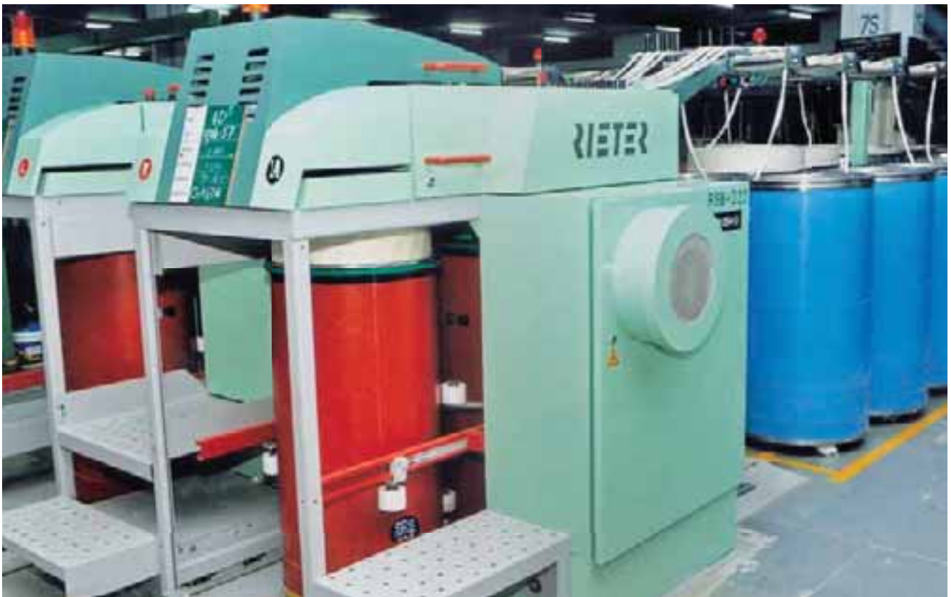
A view of the Rieter make RSB-D22 Draw Frame installed at our Textile Division, Sri Ramco Spinners, Rajapalayam
